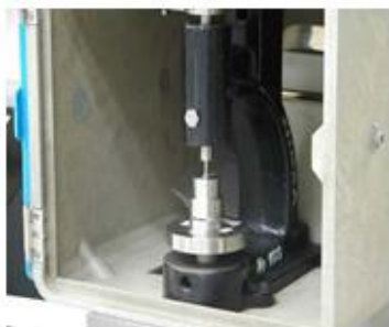
Press for the manufacture of test specimens.
