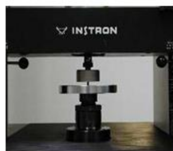
Universal Machine for compression strength test.
